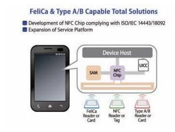
SAM: Secure Application Module; UICC: Universal Integrated Circuit Card
